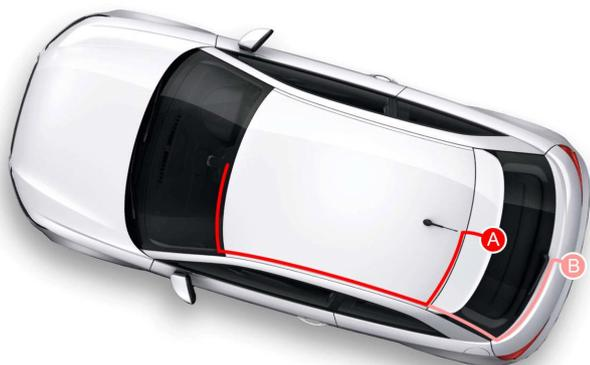
The connection cable is included. On the camera side there is a red cable that you can connect to the positive that turns on the rear lights to automatically bring the rear camera to full screen when reverse gear is engaged. If you don't want this feature you can leave the red cable unused.
