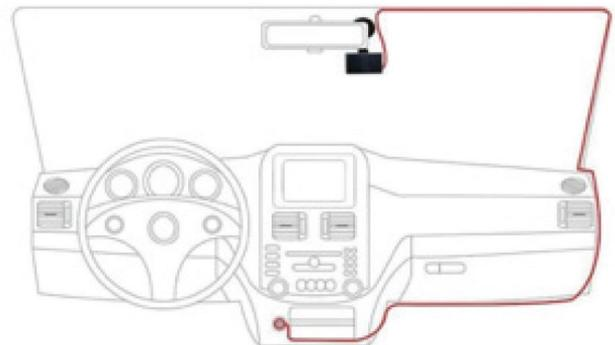
The camera should be positioned near the rear view mirror, in order to have a good front view. The best position is towards the passenger side, as shown, so as not to obstruct the driver's view.
